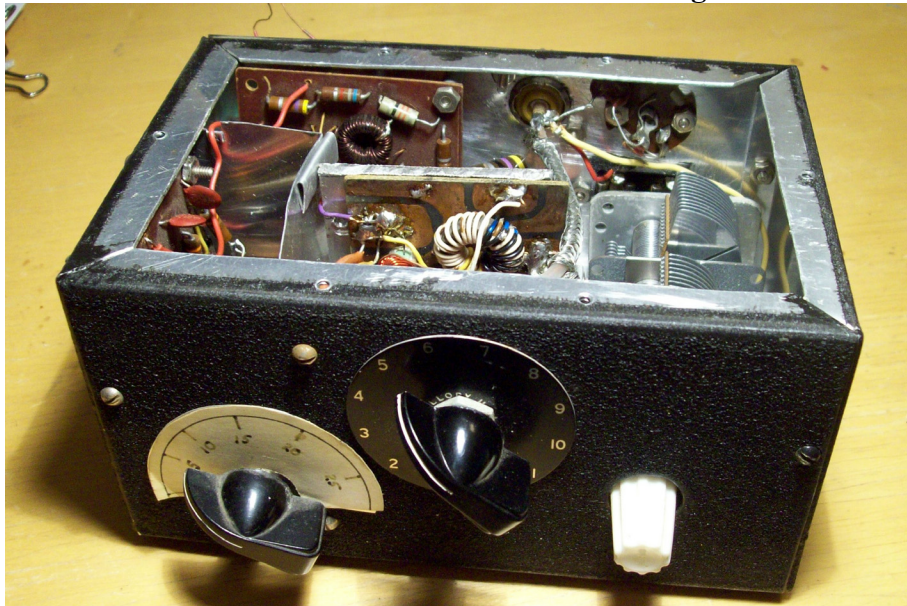
160 Meter Transmitter in Final 1975 Configuration.
